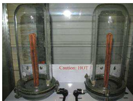
Side-By-Side Test Stand (To test untreated and treated water.)
