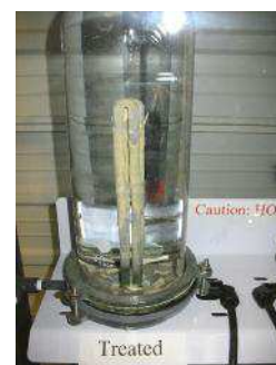
De-Scaling (After sending treated water to scaled-up heating element.)
