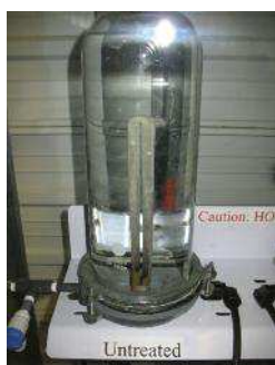
Scale Build-Up (With untreated water.)
